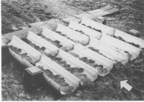
FIG. 1. Photograph of twelve paired enclosures (dimensions: 103 cm length \times 32.5 cm diameter) used to confine tailed frog tadpoles and their predators in Clearwater Creek. Arrow shows direction of flow. For each predator detection experiment (salamanders, trout, or sculpins), predators were placed in three of the six upstream enclosures; tadpoles were placed into each of the six downstream enclosures. Coarse mesh covers used to isolate predators in upstream enclosures have been removed. See text for additional details.
