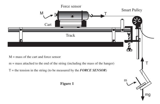
Let's apply the Work-Energy Theorem to the situation shown in Figure 1. Let M equal the mass of the dynamic cart and the force sensor, m equal the mass (including the weight hanger) attached to the end of the string, and T equal the Tension in the string (note that this Tension is measured by the force sensor). Let's agree to ignore friction and the mass of the pulley.
