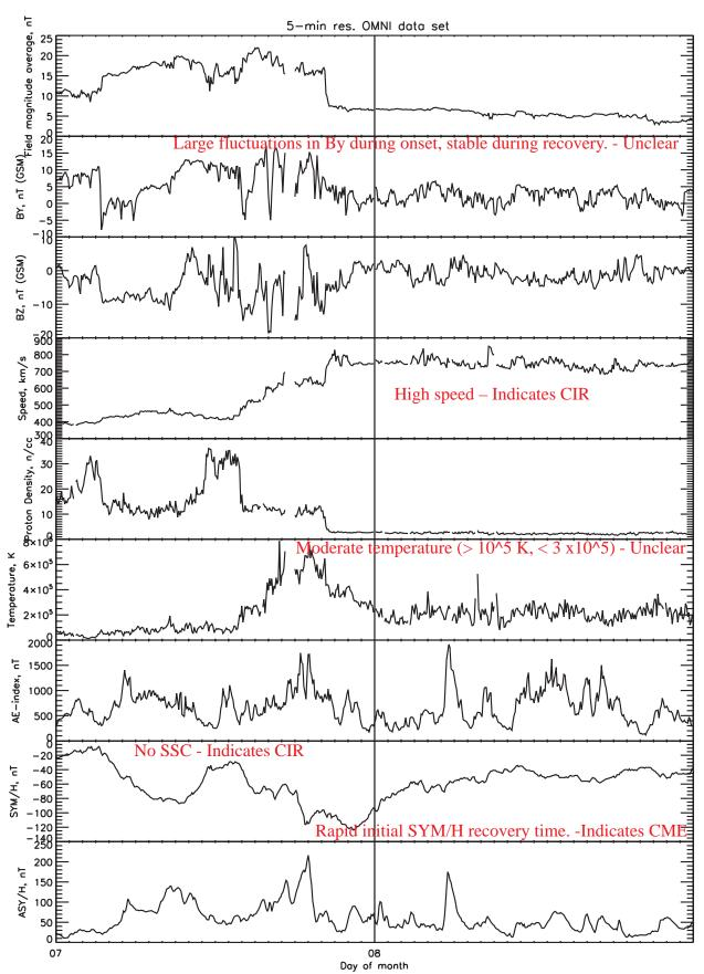
The solar wind parameters as a function of time are obtained from the OMNI web site, http://omniweb.gsfc.nasa.gov/omsc\_min.html. This data set compiled by NASA's Space Physics Data Facility includes data from ACE, Wind, IMP 8 and Geotail satellite missions. The data is shifted in time to the bow shock nose. Field and plasma parameters are determined at an appropriate time.
